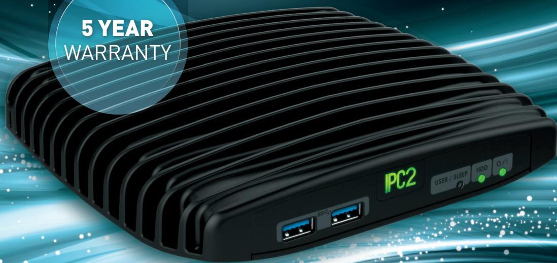
IPC2 is a miniature fanless computer based on 4<sup>th</sup> generation Intel® Core™ i7 processor. Rich functionality, connectivity and modularity, silent operation, high performance and low power consumption make IPC2 stand-out where performance, robustness and reliability matter.
